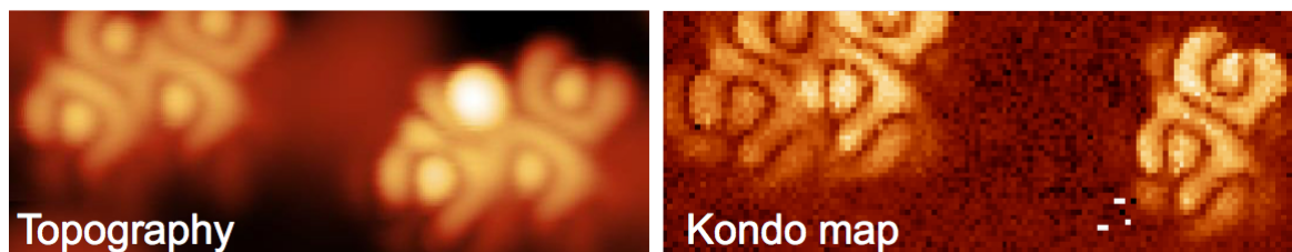
Topographic STM image of a TCNQ/TCNQ dimer and a TCNQ/TCNQ-CH 2 CN species on gr/Ru(0001) and corresponding Kondo intensity distribution map. Notice the missing Kondo signal from TCNQ-CH 2 CN.
