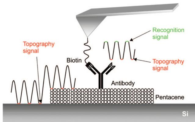
**Figure 1.** Scheme of the simultaneous topography and recognition AFM imaging of anti-biotin antibodies adsorbed on pentacene islands. A magnetically driven cantilever oscillates across the surface. The oscillation signal is split into two parts of which the lower part is used to generate the topography (topography signal, red) and the upper part is used for the recognition image (recognition signal, green).
