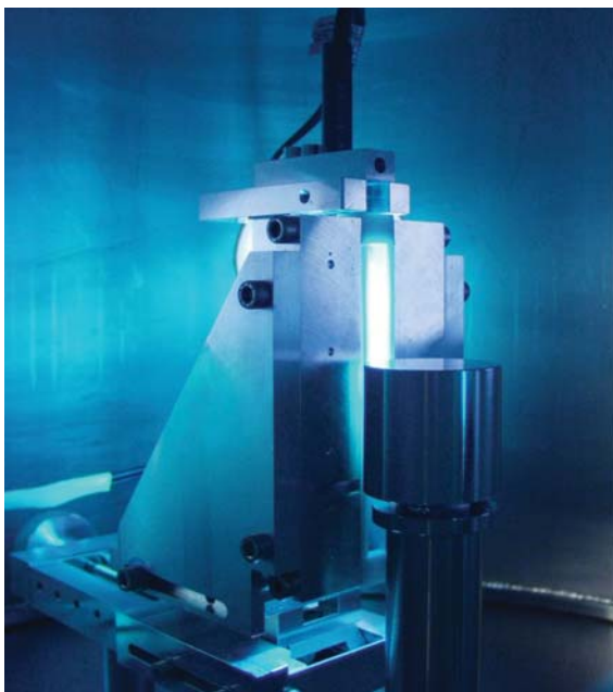
A cylindrical primary mass standard undergoes UV/Ozone cleaning
