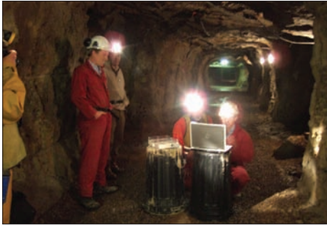
Monitoring the safety and stability of mine tunnels with networks of low-powered sensors
