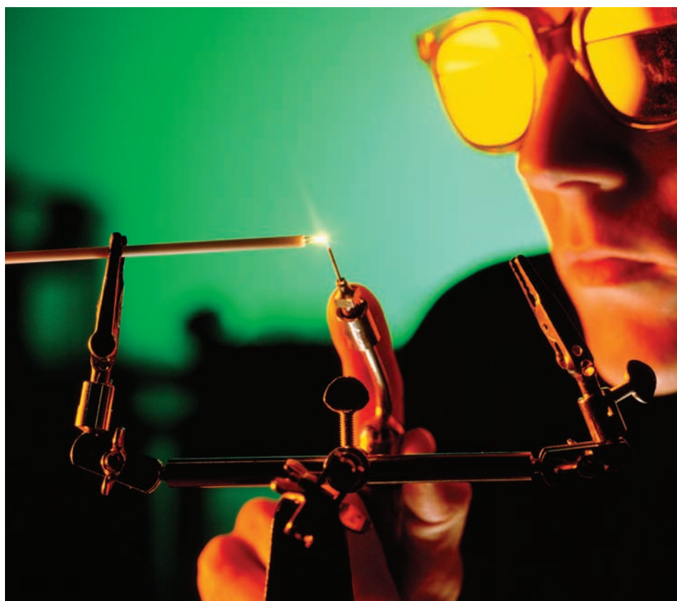
Welding thermocouple junctions using a specially designed microwelding torch
