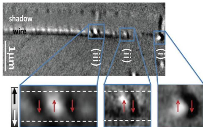
XMCD-PEEM image of a single FeCoCu nanowire with bamboo-like diameter modulations oriented perpendicular to the incident X-rays. The arrows indicate the local spin configuration, inner axial magnetization and vortex structures around the anti-notches are deduced (C. Bran et al., *J. Mater. Chem. C*, 2016, 4, 978)
