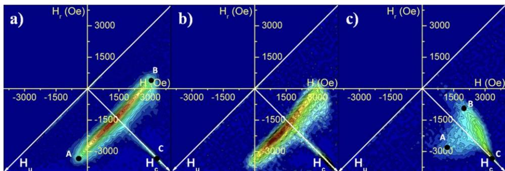
FORC distributions for FeCo/Cu multilayer nanowire arrays as a function of the Cu layer thicknesses for the same FeCo segment thickness ([FeCoCu (300 nm) / Cu(x)]<sub>10</sub>): (a) x=7 nm, (b) x=15 nm and (c) x=40 nm (E. Palmero et al. *Nanotechnology* 27 (2016) 435705).
