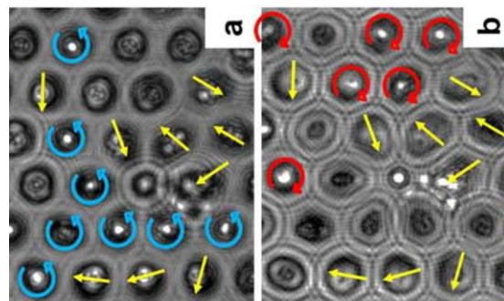
Lorentz TEM images in over- (a) and under-focused (b) conditions of an array of Co nanowires 45 nm in diameter and 55-nm long at remanence. The arrows show the transverse direction and the clockwise (red) and anticlockwise (blue) rotation of NW magnetization (Y.P. Ivanov, Y.P., Chuvalin et al. *Scientific Reports*, 6, art. no. 23844(2016))
