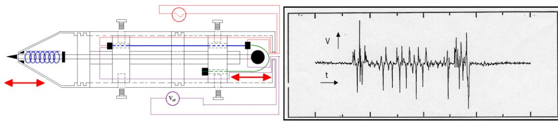
*Magnetoelastic Signature device (pen) for signature identification and authentication and magnetoelastic signature (right) using GMI effect glass-coated microwire as sensing element (Patented).*
