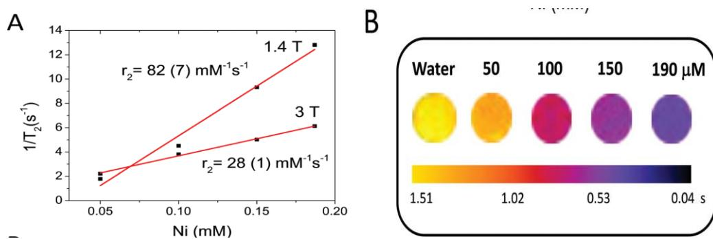
Individual Ni segments out of Ni/Cu nanowires as contrast agents for MRI imaging: Transversal relaxivity ( $r_2$ ) of a water solution of PAA-coated Ni nanowires at 1.41 T and 3 T at 37 °C (A); and  $T_2$  map of PAA-coated Ni nanowires acquired at 3 T and 37 °C (M. Bañobre-López et al., *Journal of Materials Chemistry B*, 5 (18) (2017) pp. 3338-3347)
