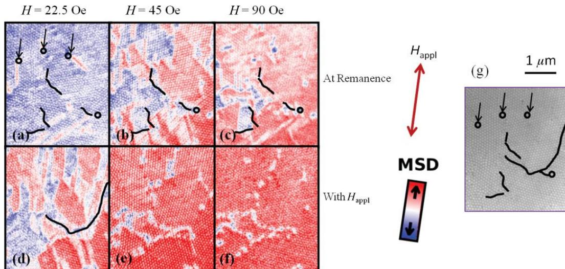
XMCD images of the magnetic domain structure of a Py antidot thin film grown on alumina template (a)-(c) at remanence and (d)-(f) under the applied field, and (g) XPEEM image denoting the geometric domains, with indication of some dislocations and punctual defects (K.J. Merazzo et al. *Phys. Rev B* 85, 184427 (2012))
