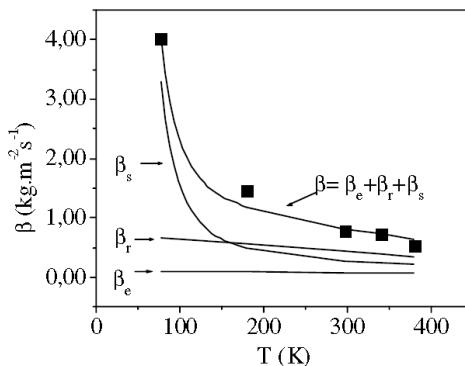
Temperature dependence of the domain wall damping  $\beta$ : experimental (square points) and calculated. Eddy current contribution,  $\beta_e$ , spin-relaxation damping coefficient,  $\beta_r$ , and structural relaxation wall damping  $\beta_s$  (R. Varga *et al.*, *Phys. Rev. Letters*, 94 (1), art. no. 017201, (2005)).
