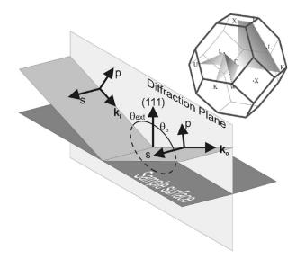
FIG. 1. Geometry of the experiment. The diffraction plane is represented in light gray. The sample surface plane is represented in dark gray. The inset shows the first Brillouin zone for a fcc structure. High symmetry points are indicated.
