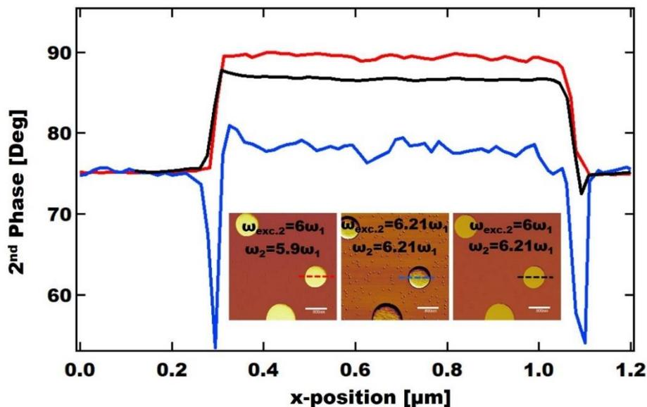
Figure 6 Phase Contrast Comparison for Different Excitation Frequencies
