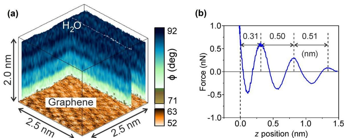
Fig 1: (a) Three-dimensional AFM image of the graphene-water interface. (b) Representative force curve obtained in close proximity to a two-dimensional material. Adapted from [4]
