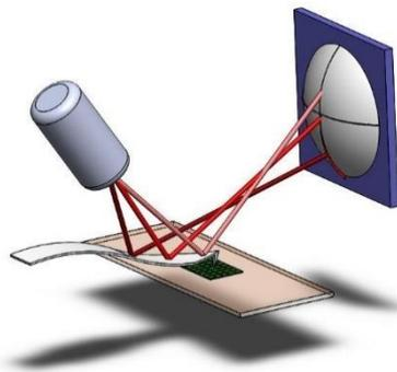
**Figure 7** Schematic of Effect of Laser Position on AFM Cantilever
