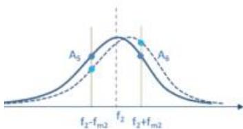
Due to the surface roughness of the BFO, single frequency resonance-enhanced PFM suffers severe instabilities, most prominent in the PFM amplitude. Imaging the sample in **DFRT-PFM** reduces the overall topographic cross-talk from step edges or dents in the sample surface significantly.
