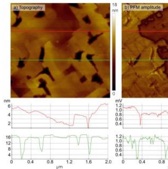
Out-of-plane and in-plane DFRT piezoresponse simultaneously captured by driving the electrical excitation of the cantilever at the contact resonance of the vertical deflection, as well as the torsional resonance on ferroelectric thin films, including bismuth ferrite and lead zirconium titanate.
