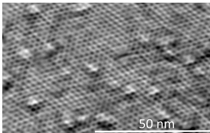
*Fig. 1: nc-AFM frequency shift image of a 120x120nm<sup>2</sup> area of a 2D polymer. Parameters:  $f_{2nd} = 1\text{MHz}$ ,  $A = 400\text{ pm}$ ,  $\Delta f_{1st} = -27\text{ Hz}$ .*
