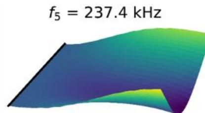
Figure 2: Simulated driven spectral response of the plate of figure 1 immersed in water.
