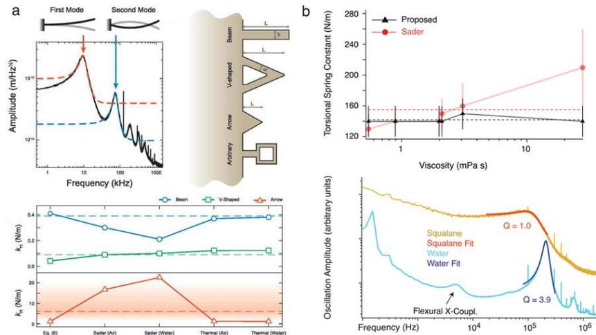
**Fig 1:** a) Calculation and comparison of the flexural spring constants from cantilever dynamics b) Comparison of torsional spring constant predictions derived with the proposed method and the Sader method in fluids of varying viscosity
