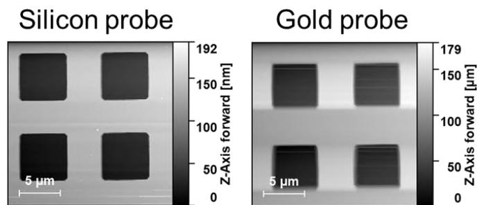
Fig 2. Comparison of LFM images obtained with commercial silicon probe and novel gold probe
