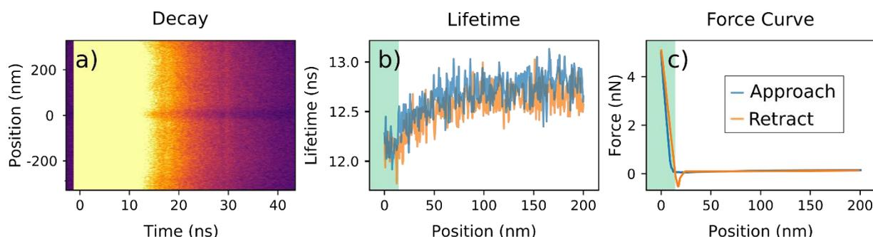
**Figure 1.** Simultaneous fluorescence decay, lifetime and force curve measurements for a nanodiamond approaching a 10 nm thick gold substrate. (a) shows all decay curves for every tip z-position, (b) shows the lifetime variations as a function of tip position, and (c) shows the force curve. In (b) and (c), blue and orange lines represent the approach and retract curves, respectively, and the light green region represents the regime of mechanical contact.
