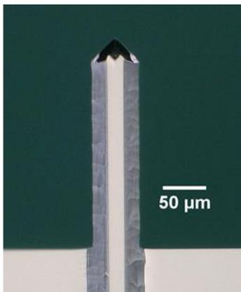
**Figure 1:** AFM cantilever used to test our model.
