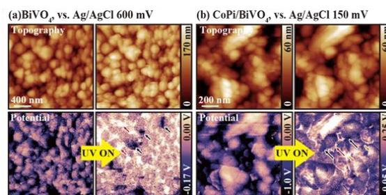
**Fig. 2:** Photo-induced changes in the topographic and potential images of the  $\text{BiVO}_4$  electrodes (a) with and (b) without CoPi cocatalysts obtained in 1 mM KCl aq. containing 10 wt.% ethanol.
