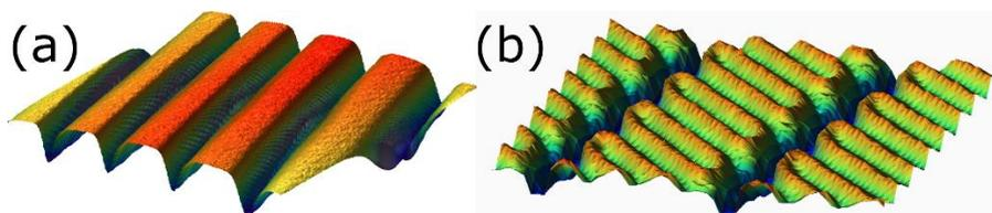
Non-contact scans in air of silicon chips provided by Applied Materials. (a) Image dimensions:  $3.6\mu\text{m}\times 3\mu\text{m}$ , Feature Height:  $16\text{nm}$ , Scan Rate:  $0.90\mu\text{m}^2 / \text{second}$ . (b) Image dimensions:  $1.5\mu\text{m}\times 1.5\mu\text{m}$ , Feature Height:  $50\text{nm}$ , Scan Rate:  $0.25\mu\text{m}^2 / \text{second}$ .
