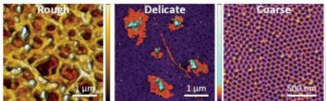
Topography images of NC membrane with a rough surface, F14H20 particles loosely bound to the surface and Al<sub>2</sub>O<sub>3</sub> aka "Tip Grater".
