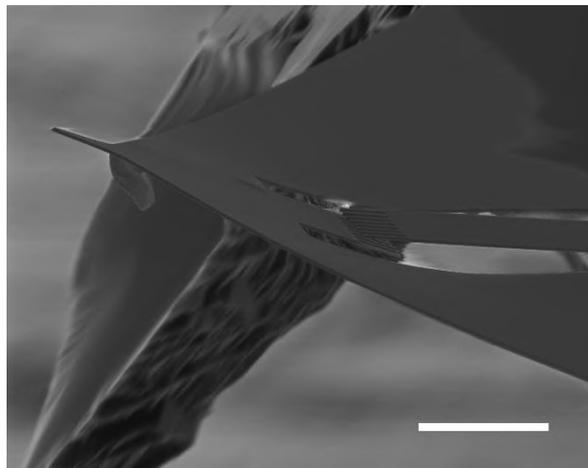
**Figure 1** – SEM image of a prototype AFM probe. The inner cantilever forms an interdigitated capacitance in series with the meander inductor. The outer cantilever carries the tip. The scale bar is 20  $\mu\text{m}$ .
