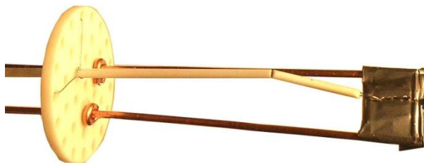
Figure 1 18: Picture of the “head” of a home-made molecular evaporator. It consists in a Ta envelope, where the molecules are deposited, which is contacted by two copper wires in order to close the circuit. Passing current through the system makes the Ta to warm up and the molecules to evaporate. A thermocouple is spot-welded to the envelope in order to monitor the temperature.
