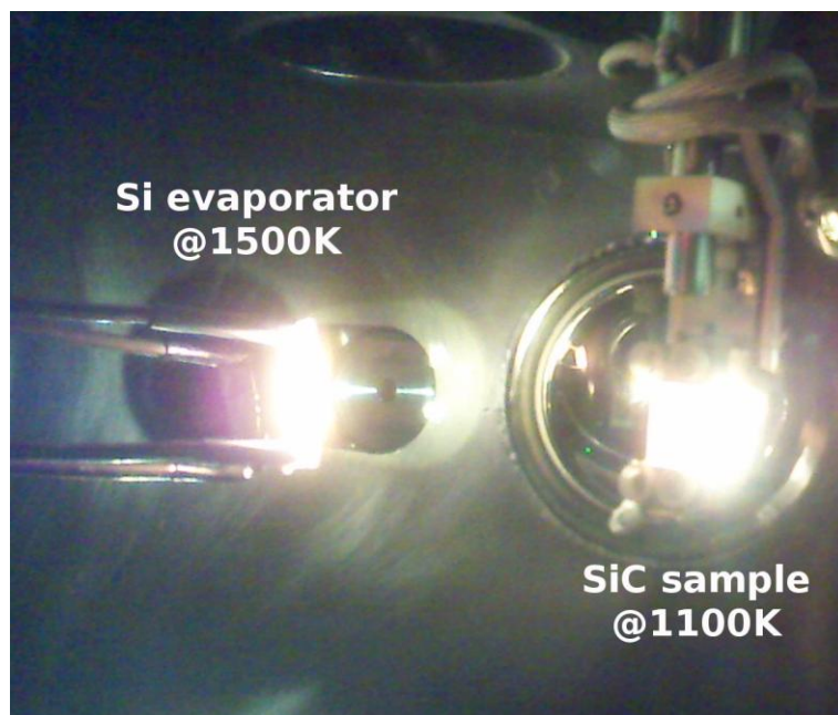
Figure 1 22: Picture of the interior of the UHV chamber during the Si evaporation and SiC treatment. The Si evaporator is placed at the left of the image whereas the sample is on the right part of the image.
